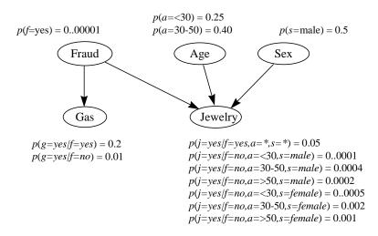
Figure 3: A Bayesian-network for detecting credit-card fraud. Arcs are drawn from cause to effect. The local probability distribution(s) associated with a node are shown adjacent to the node. An asterisk is a shorthand for "any state."
