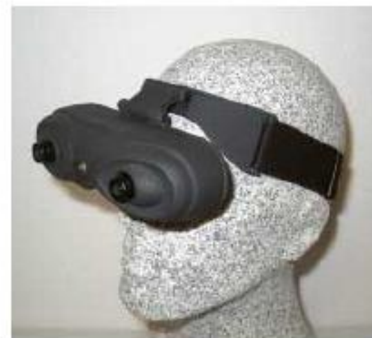
ARVision 3D HMD (commercial system) (cameras mounted over the eyes)
