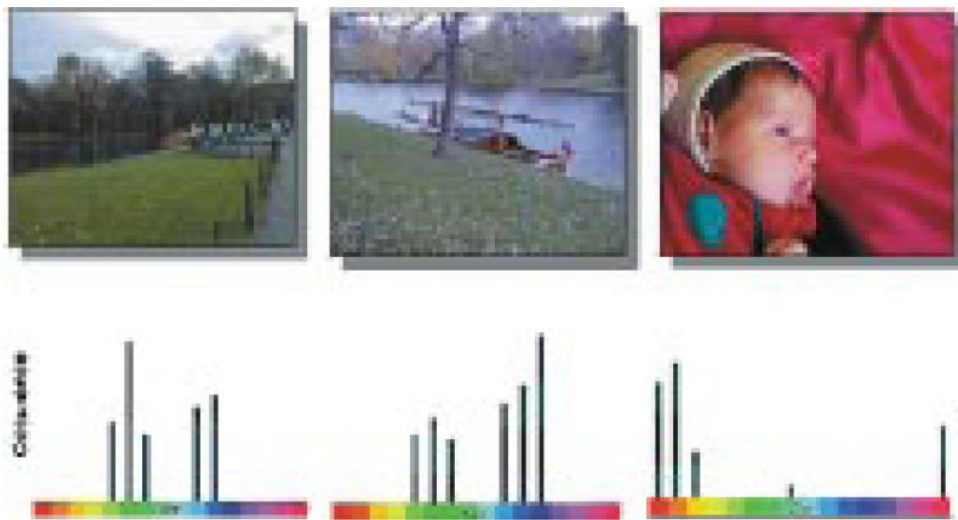
Fig. 2. Three color images and their MPEG-7 histogram color distribution, depicted using a simplified color histogram. Based on the color distribution, the two left images would be recognized as more similar compared to the one on the right.
