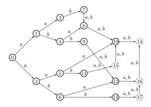
Figure 5: DFA resulting of the concatenation of DFA A with m=3 and DFA B with n=5, of Fig. 6. The states with dashed lines have level > 3 and are not accounted for by formula (1).
