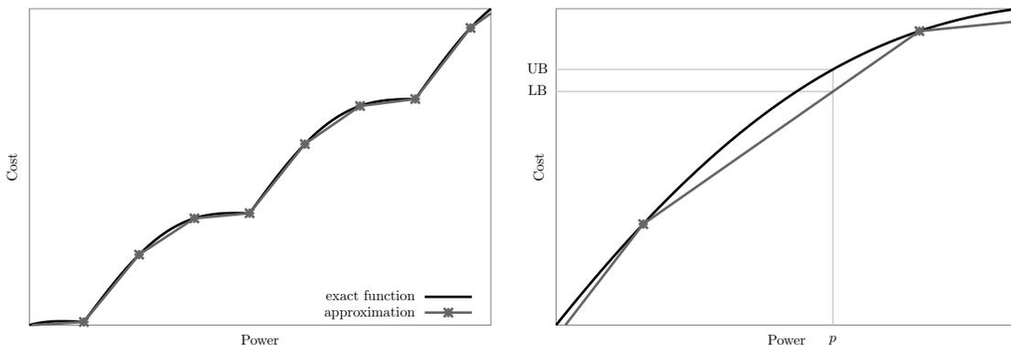
Figure 2: Fuel cost and its representation with a piecewise-linear function (left). Upper bound (UB, exact function evaluation) and lower bound (LB, piecewise-linear approximation) at a given production level  $p$  (right).
