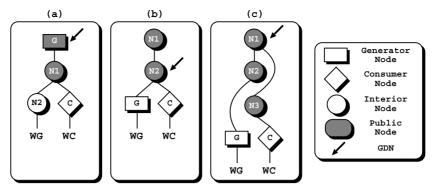
Fig. 9. Spotting the generator dependency node.
