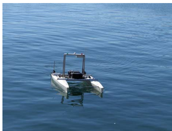
Fig. 1. The SWORDFISH Autonomous Surface Vehicle.
