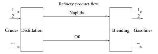
Distillation separates each crude oil into intermediate products (fractions) known as *naphtha*, *oil*, and *residue*, according to their boiling points. Naphtha and oil have octane ratings of 10 and 6, respectively. The fractions into which a barrel of each type of oil is divided can be, for example, as shown in the following table:
