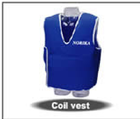
Power transmitting coil to NORIKA capsule Data receiving antenna
