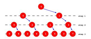
Using a tree structure for communication, we can distribute data in  $\lceil \log_2 N \rceil$  steps instead of N-1 as happened before.
