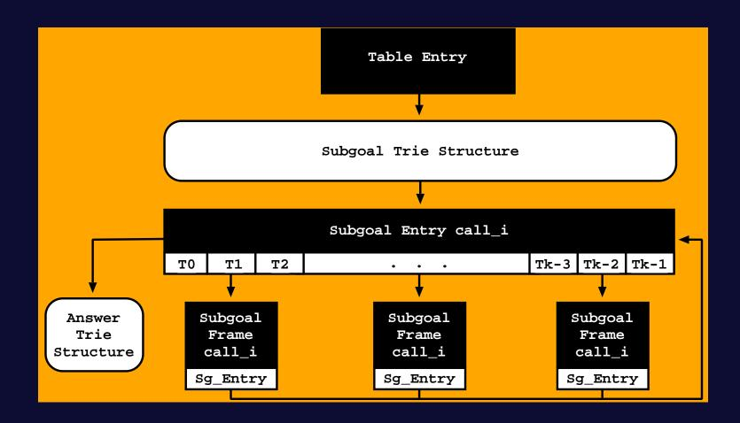
Memory usage for a table T assuming NK threads evaluating NS subgoals: sizeof(TE) + sizeof(STS) + [sizeof(SE) + sizeof(BA) + sizeof(ATS) + sizeof(SF)\* NK ] \* NS
