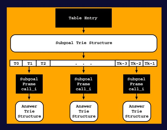
Memory usage for a table T assuming NK threads evaluating NS subgoals: sizeof(TE) + sizeof(STS) + [sizeof(BA) + [sizeof(SF) + sizeof(ATS)] \* NK ] \* NS
