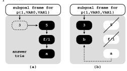
**Fig. 9.** Invalidating answers for p(X, 1, Y)(a) before and (b) after the invalidation process
