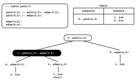
**Figure 2** An example of a tabled evaluation
