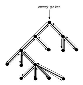
**Figure 1** Depth-first left-to-right search with backtracking in Prolog
