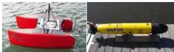
Fig. 4. Roaz ASV (left) and Isurus AUV (right)
