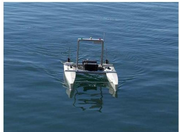
Fig. 1. The SWORDFISH Autonomous Surface Vehicle.
