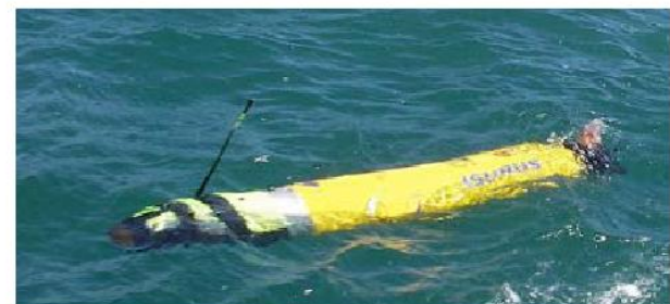
Fig. 2. The ISURUS Autonomous Underwater Vehicle.
