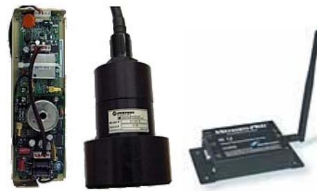
Fig. 1. Hardware: Benthos Acoustic modem (left) and transducer (middle) [3] (left) and MaxStream RF modem (right).
