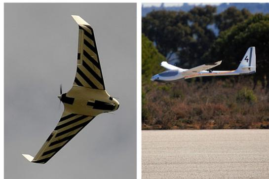
Fig. 8. ArduPilot-based MAVs integrated with the LSTS toolchain
