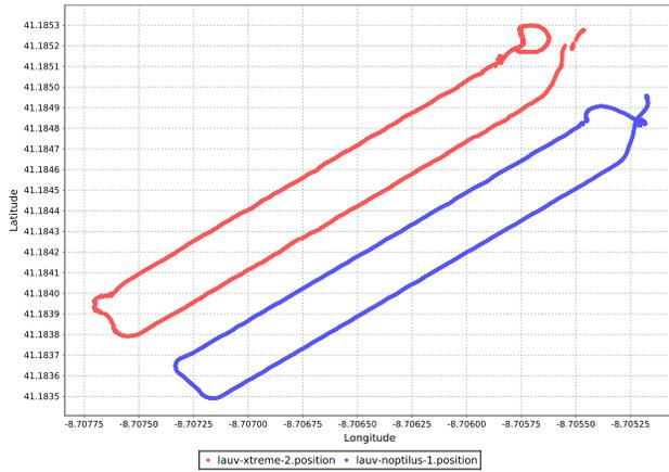
Fig. 10. Positions of vehicles in multi-vehicle survey test
