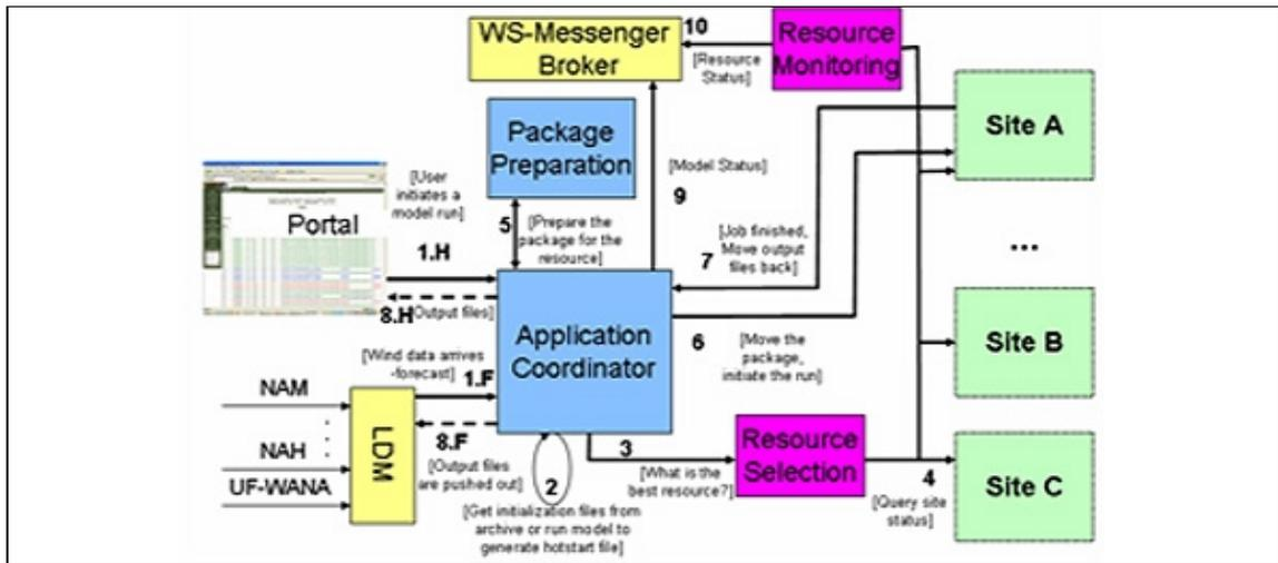
Figure CS-1. Architectural components and the control flow for the NC SCOOP system.
