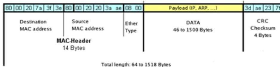
Figure NG-2. Details of an Ethernet Type II frame format.
