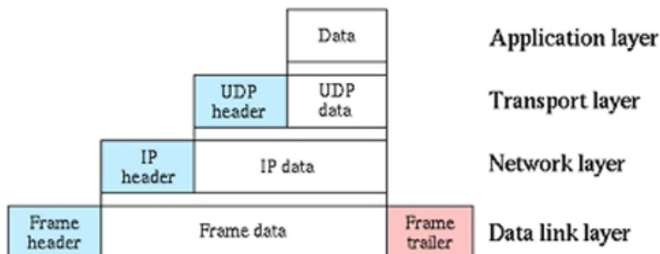
Figure NG-3. OSI data encapsulation.
