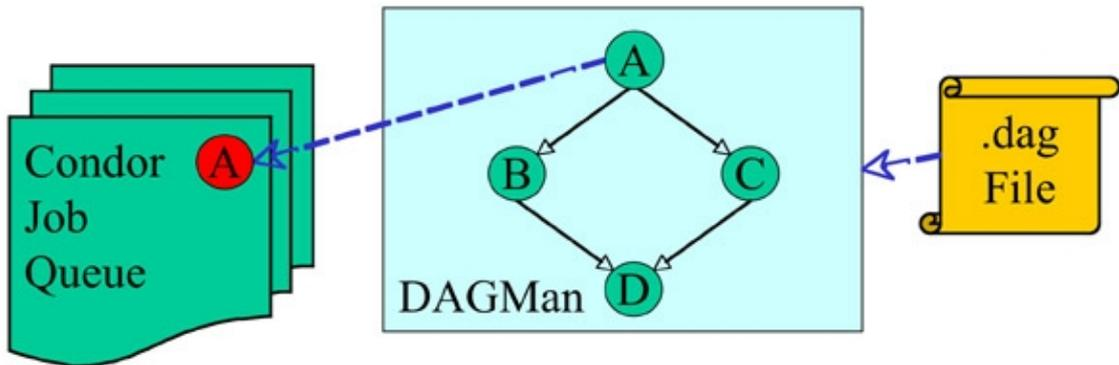
Figure PC-12. DAGman workflow diagram.
