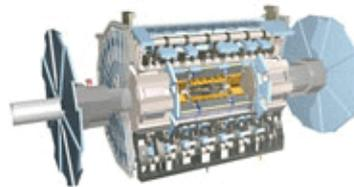
Figure CS-6. The ATLAS Detector
