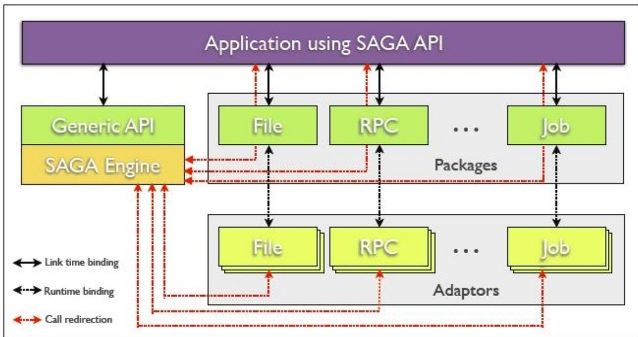
Figure PC-17. SAGA architecture: A lightweight engine dispatches SAGA calls to dynamically loaded middleware adaptors.
