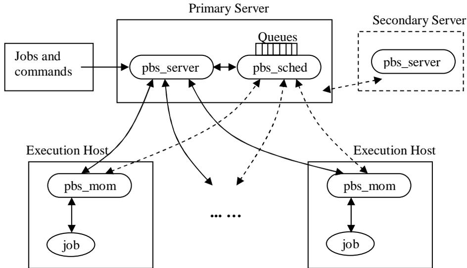
Figure 3: PBS Pro Installation Architecture
