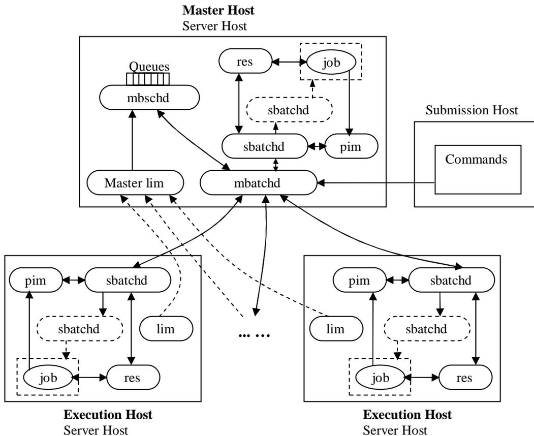
Figure 2: LSF Installation Architecture
