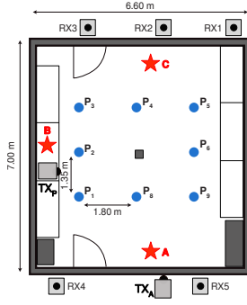
Fig. 1: Layout for the dataset in [5]. “RX” represent receiver devices, “TX P ” and “TX A ” are passive and active attack transmitters, stars “A”, “B”, and “C” are possible obfuscator positions. P_1 to P_8 denote the 8 prospective user locations.
