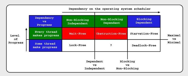
Obstruction-free (a thread runs within a critical region in a bounded number of steps) requires the OS scheduler to allow each thread to run in isolation for a sufficient amount of time (non-blocking dependent).
