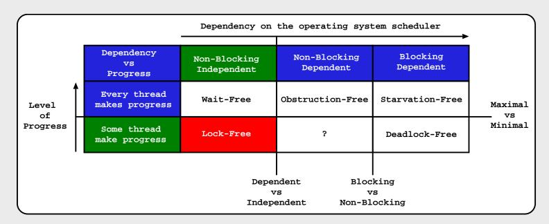
Lock-free provides minimal progress and has no requirements on the OS scheduler (non-blocking independent).
