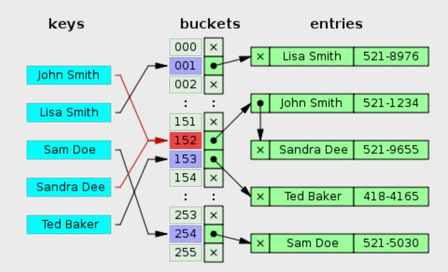
Key collisions resolved using a separate chaining mechanism [Wikipedia].
