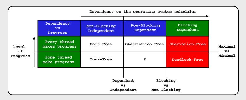
Deadlock-free (threads cannot delay each other perpetually) and starvationfree (a critical region cannot be denied to a thread perpetually) properties guarantee progress, however, they depend on the assumption that the OS scheduler will allow each thread within a critical region to be able to run a sufficient amount of time, so that it can leave the critical section (blocking dependent).
