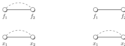
Fig. 11.9. The equality graph corresponding to Example 11.31 obtained with Ackermann’s reduction ( left ) and with Bryant’s reduction ( right )
