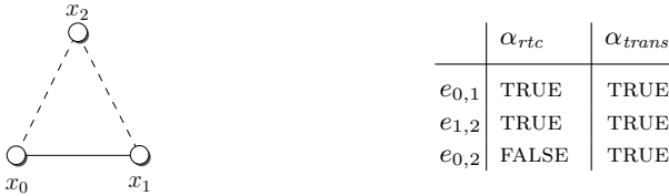
Fig. 11.10. Taking polarity into account allows us to construct a less constrained formula. For this graph, the constraint \mathcal{B}_{rtc} = (e_{0,2} \wedge e_{1,2} \implies e_{0,1}) is sufficient. An assignment \alpha_{rtc} that satisfies \mathcal{B}_{rtc} but breaks transitivity can always be “fixed” so that it does satisfy transitivity, while still satisfying the propositional skeleton e(\varphi^E) . The assignment \alpha_{trans} demonstrates such a “fixed” version of the satisfying assignment
