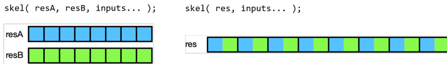
Fig. 2: Difference in return value storage between using multi-valued return (left) and single-value (by manually managed array-of-struct) return (right).
