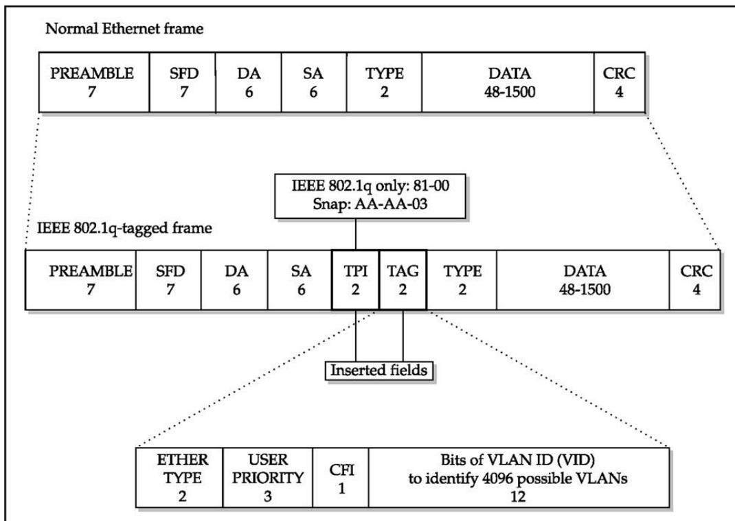
Figura 5 — Encapsulamento 802.11Q vs. *ethernet* normal
