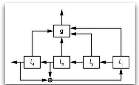
The g function must be a nonlinear function—one that both XORs bits together and combines them with logical AND or OR operations.
