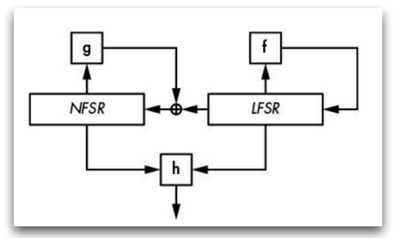
Grain-128a combines a 128-bit LFSR, a 128-bit NFSR, and a filter function, h. The LFSR has a maximal period of  $2^{128} - 1$ , which ensures that the period of the whole system is at least  $2^{128} - 1$  to protect against potential short cycles in the NFSR. At the same time, the NFSR and the nonlinear filter function h add cryptographic strength.
