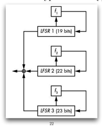
How could this be seen as secure with only LFSRs and no NFSR? The trick lies in A5/1's update mechanism. Instead of updating all three LFSRs at each clock cycle, the designers of A5/1 added a clocking rule that does the following:
