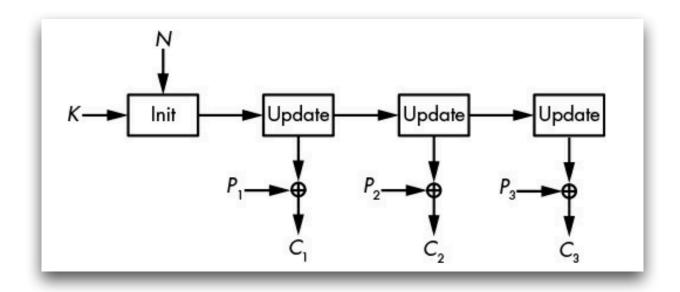
The cipher initialises the state from the key and the nonce and then calls an update function to update the state value and produce one or more keystream bits from the state.
