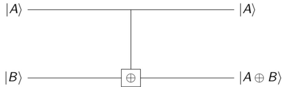
The first particle acts as a conditional to change the state of the second. The circuit is equivalent to
