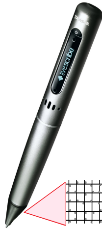
Fig. 3. Livescribe Smartpen and the dotted position system
