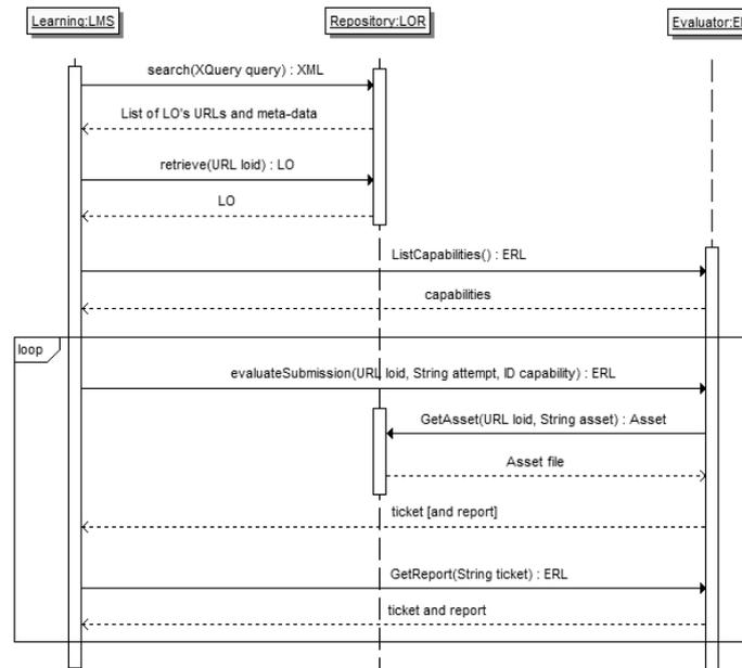
Fig. 1. Interacting with the evaluator.
